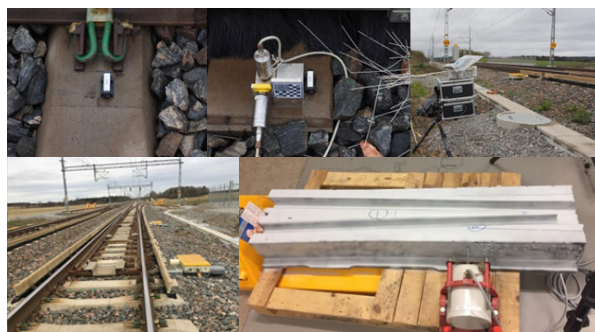
Figure 1 - In order from top left; MEMS accelerometer, Geophone, High Speed Camera, Algutsgården site and Acoustic Emission laboratory trial
