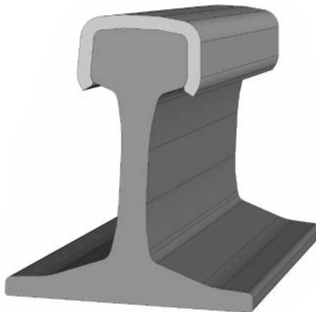
Figure 12.12: Illustration of a rail with a replaceable head
